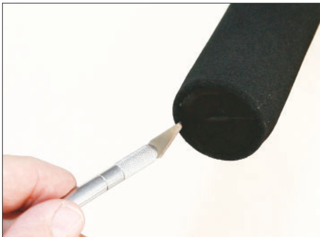
The throttle control fits into the end of the handlebar, so you need to cut a hole in the end of the grip.
