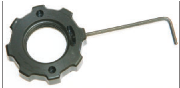
The tension on the hand wheel is adjusted by way of a small setscrew. We found the adjustment was right to our liking.
