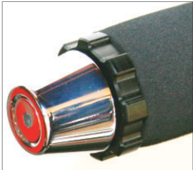
The finished installation. When the hand wheel is rotated, it locks the throttle grip.
