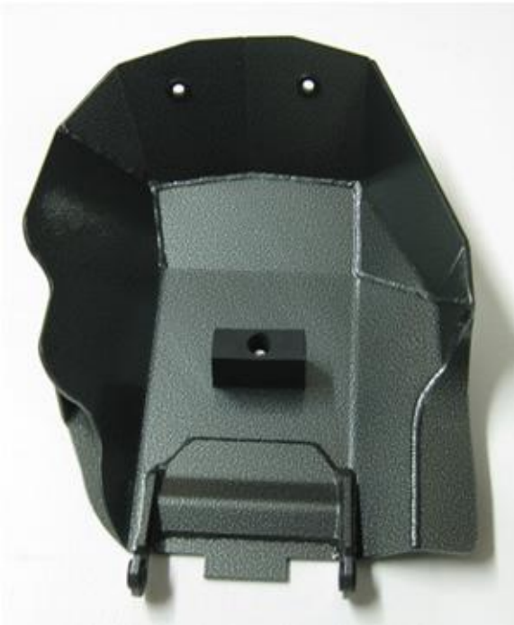
Correctly installed "Shok Blok" bumper
