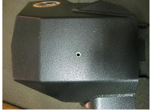
Countersunk hole in bottom of skid plate
